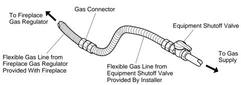
Figure 25 - Attaching Flexible Gas Lines Together
